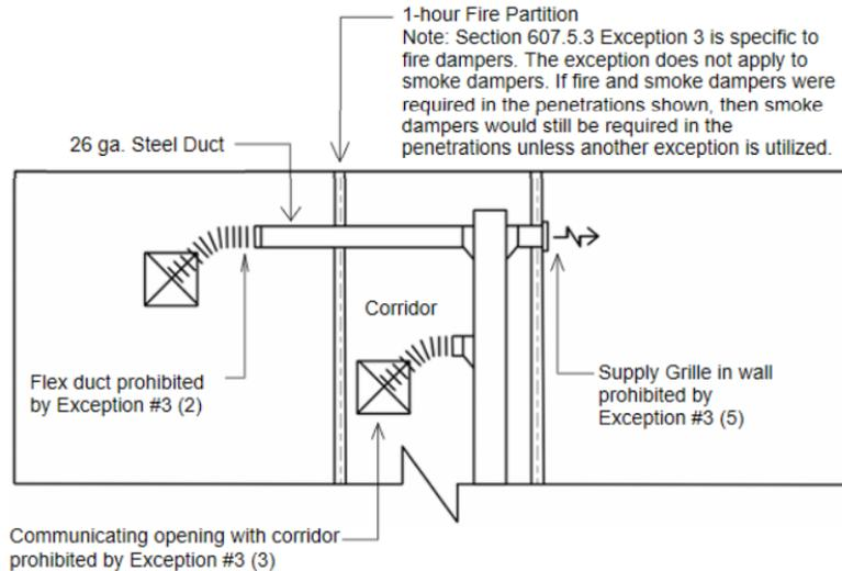
*Example 3: An unsprinklered building. The design shown is not compliant with NCMC Section 607.5.3, Exception 3, as there are communicating openings in the corridor, the flex duct does not meet the material requirements, and the duct terminates at a wall register.*
