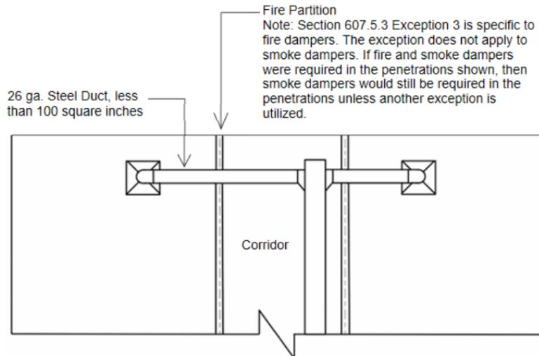
*Example 2: An unsprinklered building. The design shown is compliant with NCMC Section 607.5.3, Exception 3. The duct penetrating the wall meets the requirements of the exception and there are no communicating openings with the corridor.*
