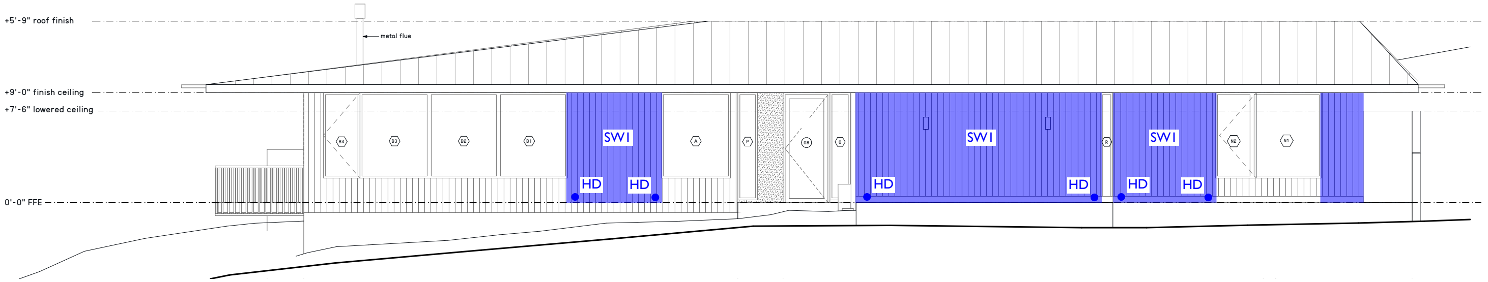
03 SOUTH ELEVATION SHEAR WALL LAYOUT
