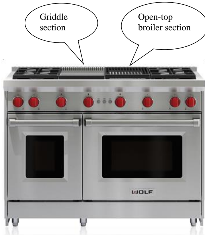
Figure 3: Domestic appliance with open-top, under-fired gas broiler. It also has a griddle. This appliance does require a means of exhaust due to the presence of the open-top under-fired gas broiler, per NCFGC 623.5. (Wolf-SubZero, 2017)
