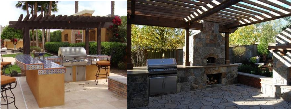
Figure 2: Pergolas, combustible structures – These are also not outdoors
