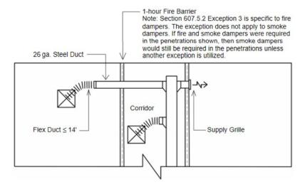
Example 1: A fully ducted system in a fully sprinklered building where the only flexible duct in the system is used to connect the air terminal to the system after the 26 ga. duct penetrated the 1-hour fire barrier. The design shown is compliant with NCMC Section 607.5.2, Exception 3.
